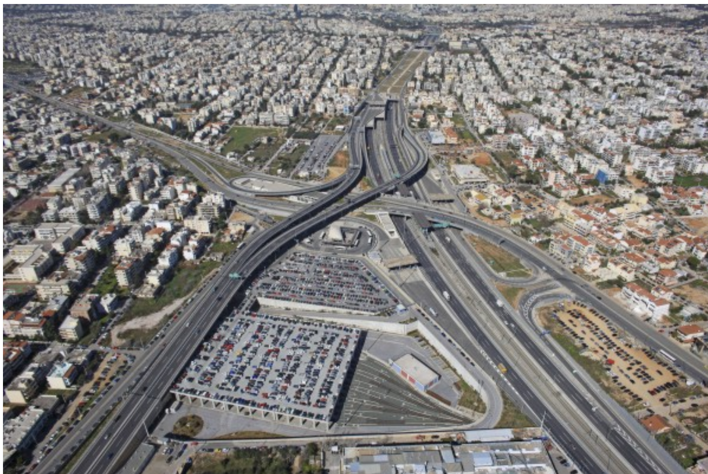
Plakentias interchange and multimode transfer facility, including 5-leg interchange, metro station, suburban railway station, bus terminal and Metro line 3 depot, Greece.
